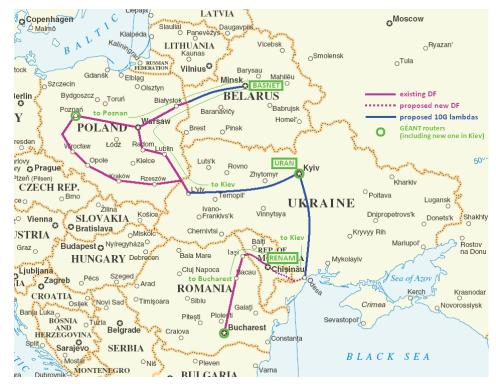
Figure 3. Geographical scheme of EaP North to South optical arc implementation
